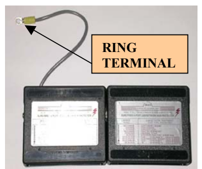
TOP VIEW WITH HORIZONTAL STACK & GROUND WIRE
