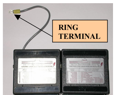
TOP VIEW WITH HORIZONTAL STACK & GROUND WIRE
